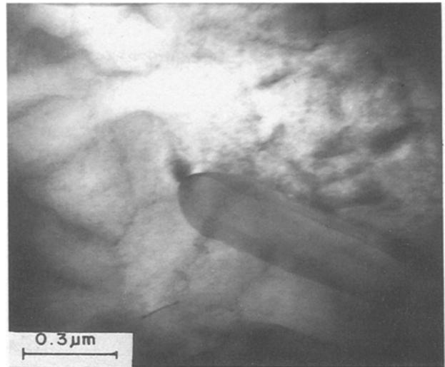
Figure 7 Transmission electron micrograph of as-spun Bi-6 wt % Mn alloy.
